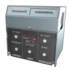
Solid State Pressuretrol with line voltage pressure controller that provides automatic operating control, automatic limit protection, manual reset limit protection, and 4-20ma modulating firing rate control for pressure systems up to 300 psi.
