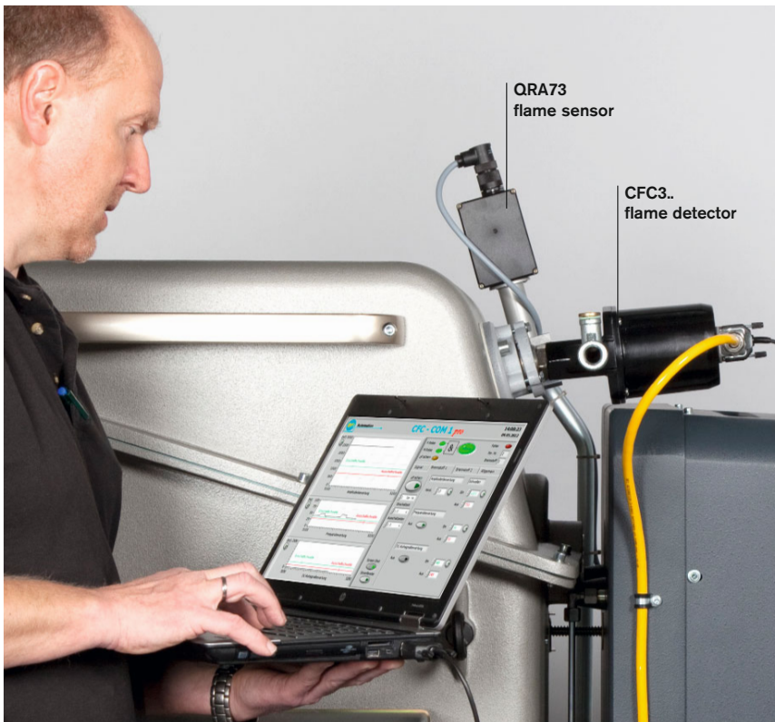
Testing and optimisation using a software tool
